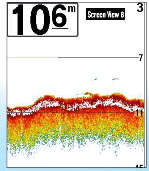
signal shows two different bottom surfaces. Notice in the left part of the recording the bottom echo signal is thick, indicating a hard raised bottom surface, where rocky outcrops, crevices and ledges potentially exist. Now notice in the right section of the recording the bottom echo signal is thin, indicating this section of the bottom has a flat surface, typically a sand bottom, which produces a thinner bottom echo signal because it has a soft reflective surface.
