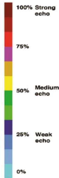
The images of fish and bottom structure recorded on the display are recorded in many different colours according to their signal strength, also known as target strength.
