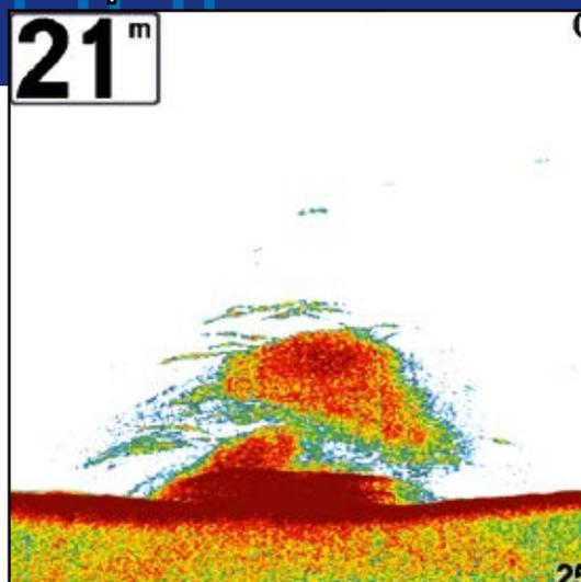
shape and the flesh density is similar to that of water. Therefore the gas content and volume of the swim bladder significantly contributes to the amount of acoustic energy reflected from the fish. Large fish such as dhufish have high target strength and produce a stronger echo signal because they have a bigger mass, have a large swim bladder, bigger bone structure and will have large, heavy scales. Smaller fish have lower target strength because of their smaller size and structure.
