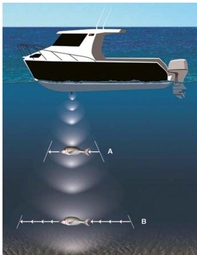
Since the maximum intensity of the sound waves is concentrated in the centre of the beam as shown in figure (Three), fish targets detected in the beam at A will be recorded as a stronger colour than similar fish detected on the outer limits of the beam at B. Therefore, a large fish detected at the edge of the beam will be recorded as a much weaker signal than if it had been detected in the central axis of the beam
