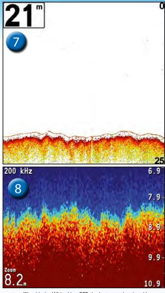
capture (8), with the White Line OFF, the bottom echo signal has been zoomed and shows an image of a bottom covered in seagrass.
