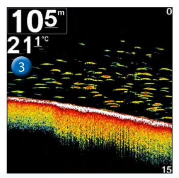
no marine plant life visible above the White Line in this image. Echo signals from large individual fish targets can be seen throughout the water column.
